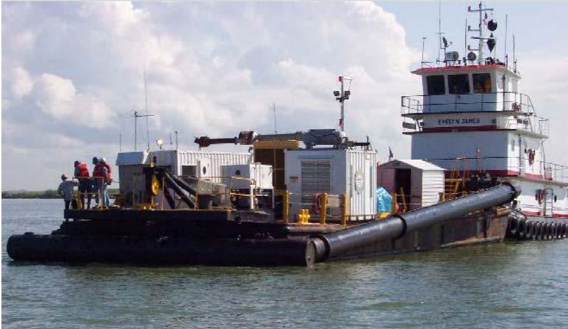
Figure 3b. The Weeks Marine, Inc. water injection dredge, Weeks Marine BT 773 (Schroeder et. al, 2018).
